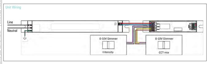
Note: Dimmers to be provided by others. Tunable White and Tunable Green to White configurations require dimmers for both intensity and color temperature.
